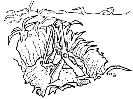
Figure 8. (a) The scissor-jawed trap is set so that the jaws straddle the runway.
